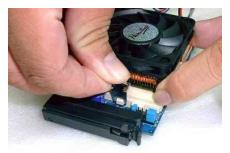
Attaching the heatsink/fan's retaining clip to the ZIF socket. (2)
